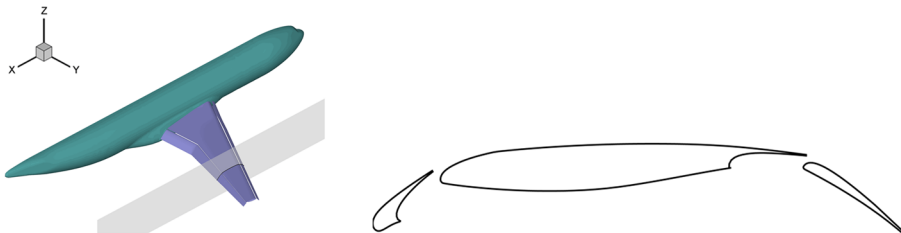
Fig. 1 Wing section of the KH3Y model in landing configuration at the location of pressure row DV06.
